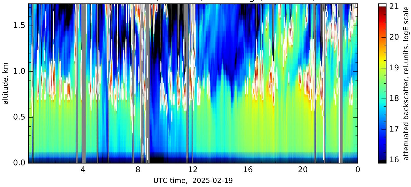
Particle backscatter, 532nm, complete range, res.: 120s, 60m-660m
