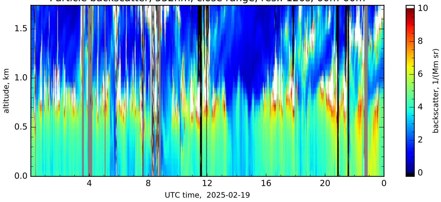
Particle backscatter, 355nm, complete range, res.: 120s, 60m-660m
