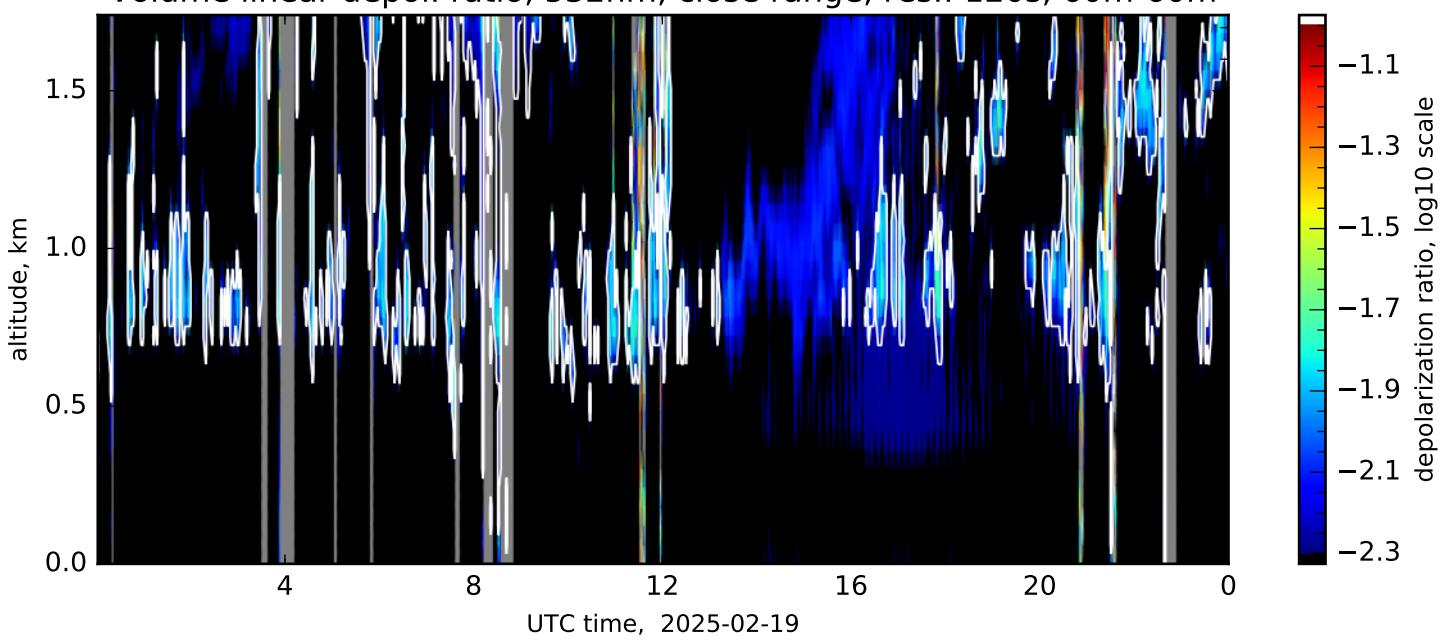
Particle linear depol. ratio, 532nm, complete range, res.: 120s, 60m-660m
